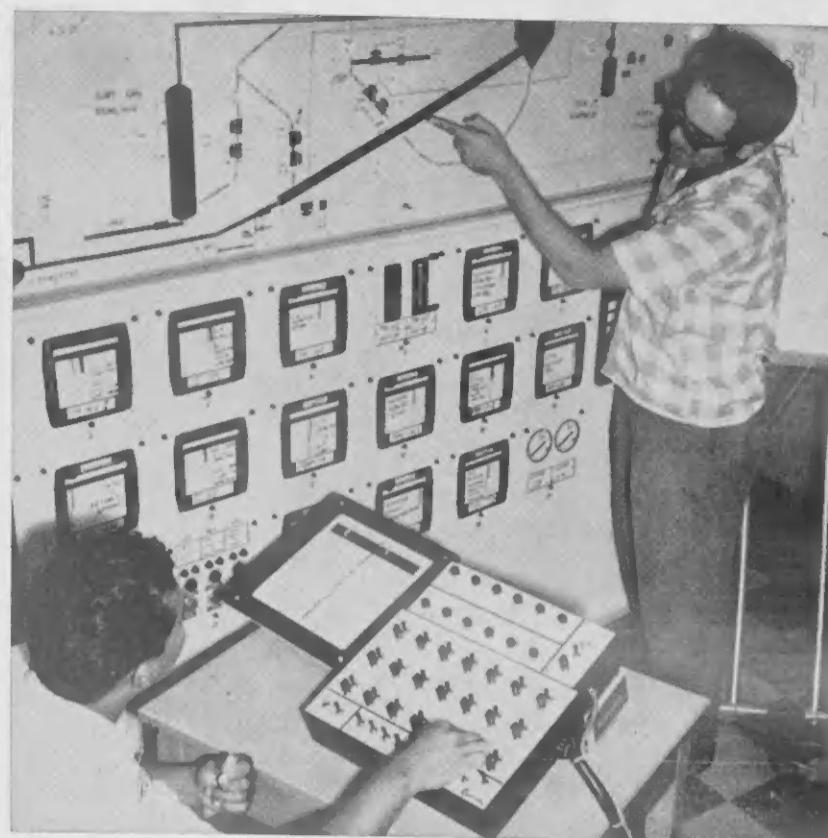
CARMODY TRAINING instructor F. Maduro at remote-control console directs B. Croes, a Process employee, on the operation of the Cat Cracker.
